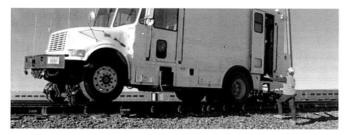
Using the latest customized ultrasound technology, railroads are detecting microscopic flaws in steel rail track before they cause accidents. Railroads are focusing intently on track safety because faulty track is a leading cause of accidents.
