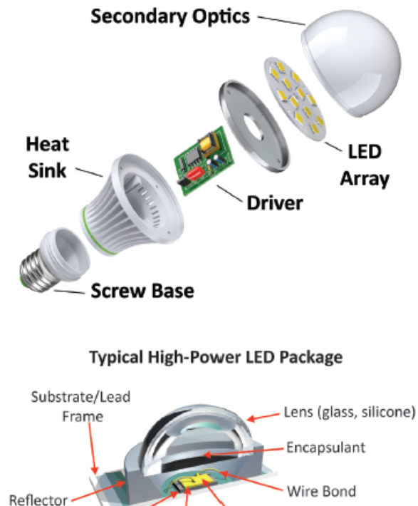
Figure 4. Elements of an LED package and typical LED lamp. Source: IES 2020.
