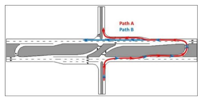
A J-Turn, or reduced conflict intersection, is a u-turn type intersection installed on divided highways (expressways). A J-Turn requires vehicles on the side street intending to cross a divided highway or make a left turn onto the divided highway to use the u-turns installed in the divided highway median. Vehicles on the divided highway can still make a left turn or right turn at the intersection as normal.
