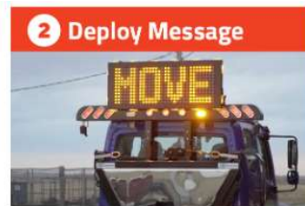
Deploy the sign using the pair tablet or SafeAll Sign Dial. Easily change messages by using the Quick Links menu on the tablet or Sign Dial.
