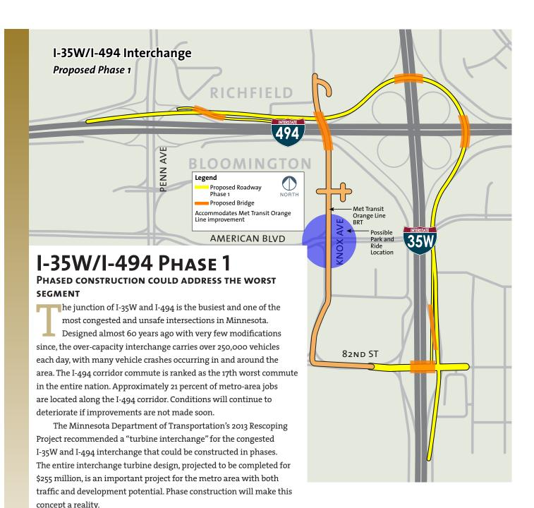
Phase 1 interchange improvements would include making temporary lanes to accommodate rerouted traffic, rebuilding of the 82nd Street bridge over I-35W, and constructing access from north-bound I-35W to west-bound I-494. This portion of the Phase 1 project is estimated to cost \$85 million. Timing construction to coincide with Metro Transit's Orange Line Bus Rapid Transit work in 2018-2019 will minimize construction costs and delay to the public.
