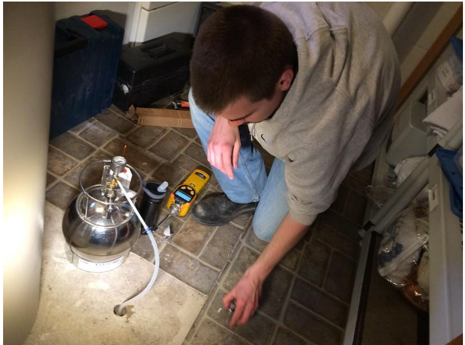
Testing for the presence of harmful soil vapors under a basement floor at a site in St. Louis Park.
