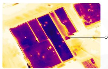
There is energy loss showing in the roof, this could possibly be from a lack of insulation.
