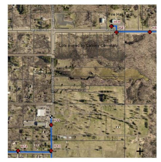
• Approximate extension 3,400 feet connecting Hydrant 47 to Hydrant 11
