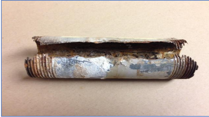
Failed Galvanized Waste Pipe
