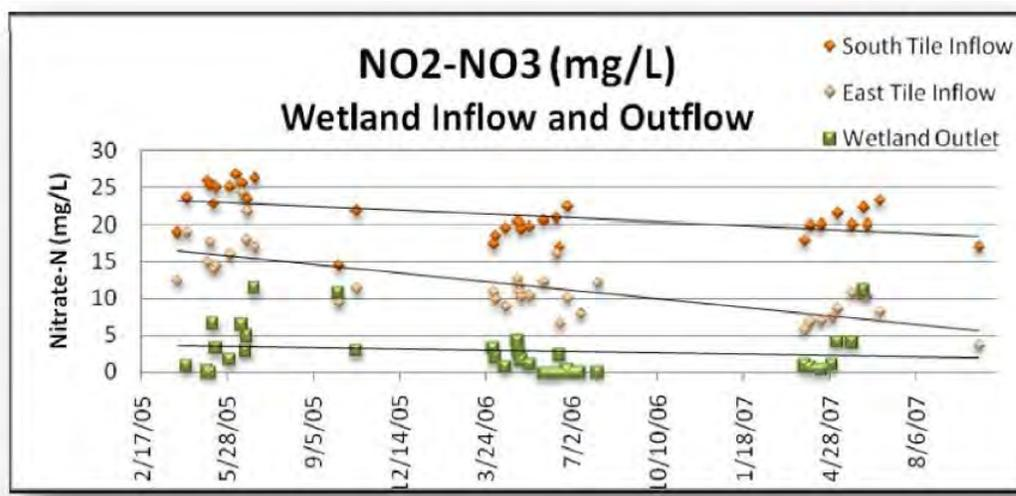
Figure 33. Inlet and outlet  $\text{NO}_x\text{-N}$  concentration for County Ditch 58 constructed wetland, located in Seven Mile Creek watershed in Minnesota, from 2005 to 2007. East tile inflow was treated by another upstream constructed wetland prior to the County Ditch wetland. Reprinted from Kuehner (2009).
