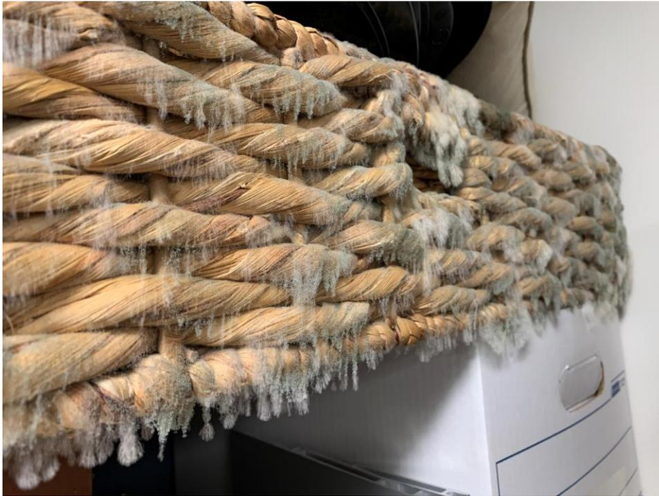
Mold growth in a basement area converted and used as staff office space with inadequate ventilation and high humidity levels
