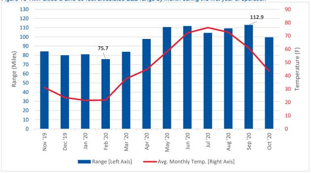
Figure 18 Twin Cities C Line 60-foot articulated BEB range by month during the first year of operation<sup>43</sup>
