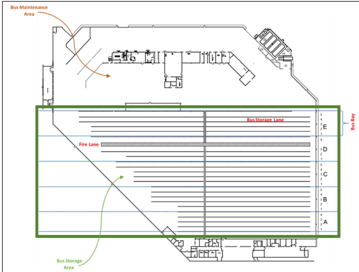
As BEBs are typically the same length as conventional buses, impacts to bus storage capacity associated with electrifying a garage are primarily due to the spatial requirements of the chargers themselves. To model these spatial impacts on bus parking capacity at each garage, two factors must be considered:
