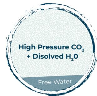
*Historically, CO<sub>2</sub> pipelines have transported relatively dry and pure CO<sub>2</sub>. However, the expansion in different sources of CO<sub>2</sub> has the potential to lead to higher water content and more impurities introduced into pipelines. In addition, carbon dioxide mixed with water can form carbonic acid which is extremely corrosive to the internal surface of the pipe.*
