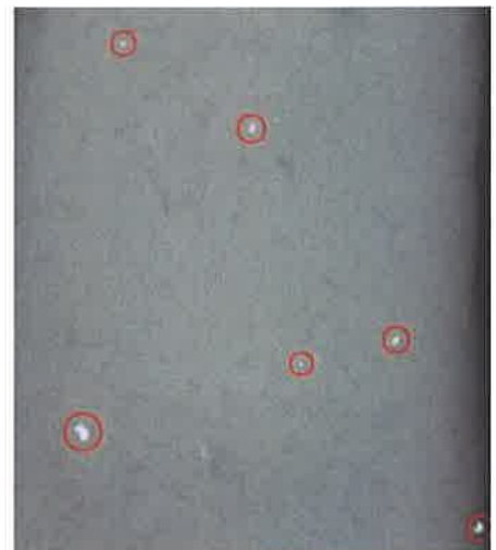
X-ray of a package of processed venison, lead fragments are circled in red. | nps.gov
