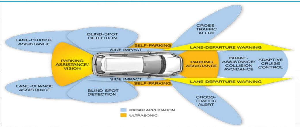
Figure 2 Several driver-assistance systems are currently using radar technology to provide blind-spot detection, parking assistance, collision avoidance, and other driver aids (courtesy Analog Devices).
