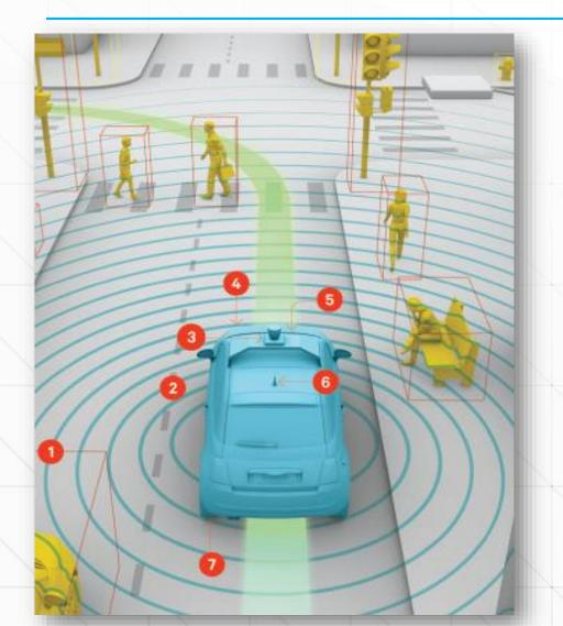
**1. Radar:** Detects objects nearby & in "blind zones" 2. Lane-keeping Cameras: Measures contrast between road and lines 3. LIDAR: Spinning lasers make a 360° realtime "map" around vehicle 4. Infrared Camera: Detects objects ahead in the day & night 5. Visible Light Camera: Detects & predicts movement of objects 6. GPS Navigation: Advanced mapping tells the vehicle where to go 7. Wheel-mounted Sensors: Measures velocity relative to close objects
