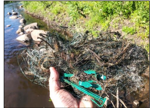
Plastic erosion control blanket.
