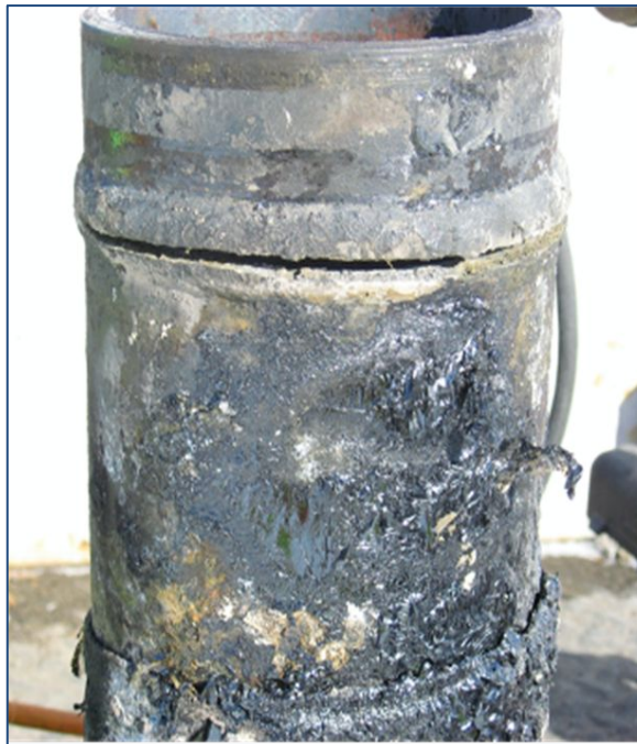
Left: Morris Campus - ruptured natural gas pipe
