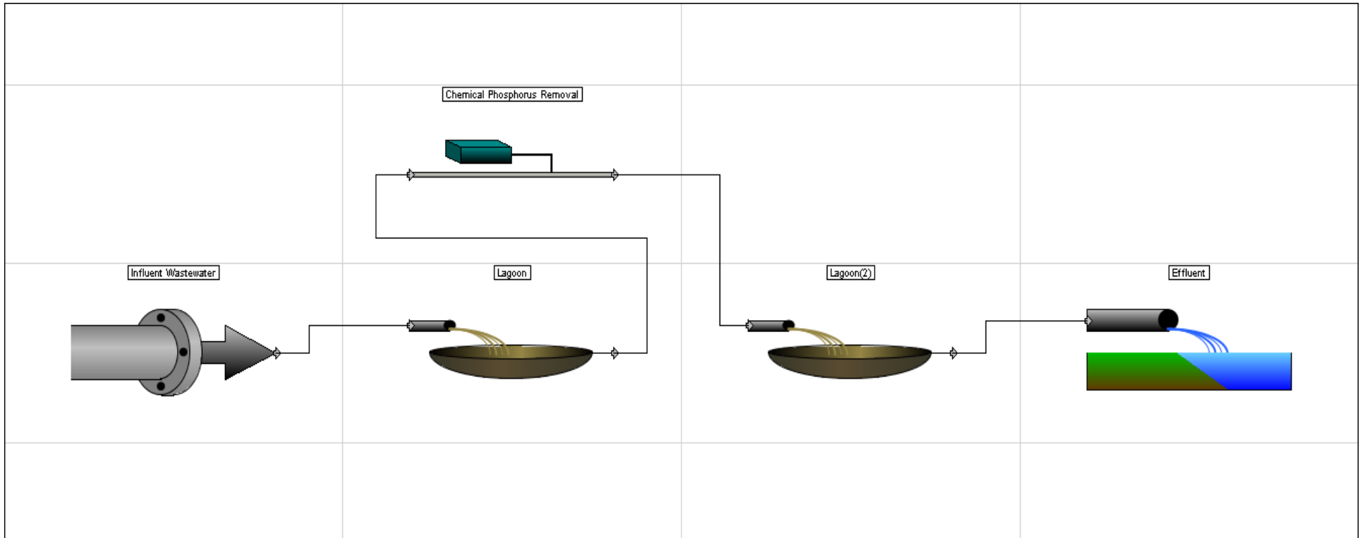
Figure D-2 Process flow diagram of potential WWTF upgrades to meet existing permit limits for Hanska
