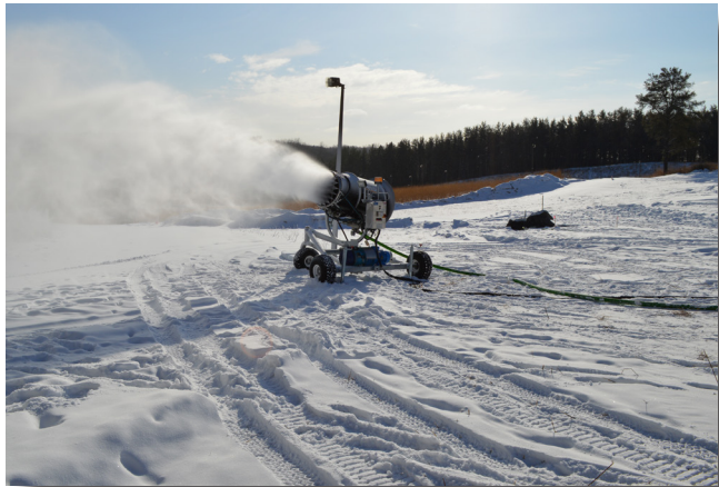
Portable snowmaking guns demonstration at Battle Creek Regional Park. Portable snow guns are used to establish cross country ski trails.
