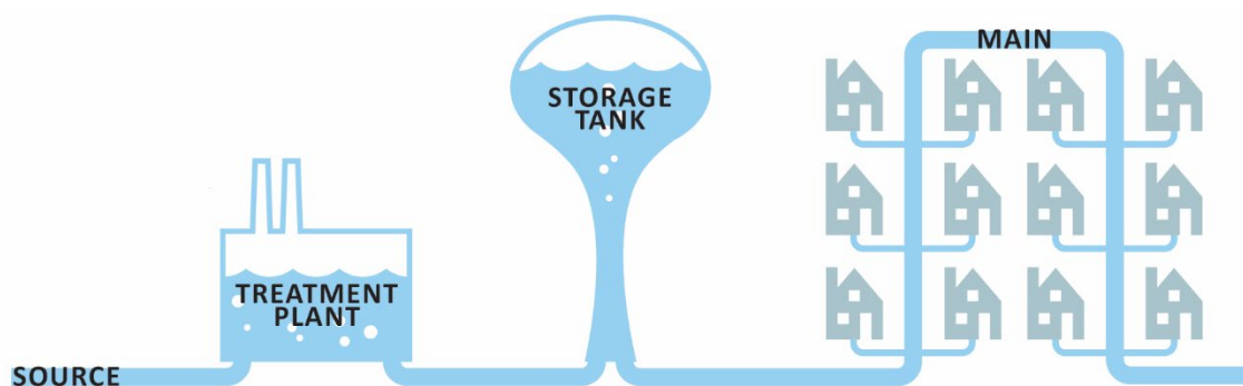
Figure 5: Water Supply Distribution System
