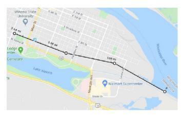
Upgrade an existing siding track with power switches and signals to allow more efficient train meets and the ability to clear the main track more quickly and efficiently; improve safety for passengers who can board the train from the track adjacent to the platform instead of walking across tracks. Note: The Winona Station platform will be improved by Amtrak through a separate project.
