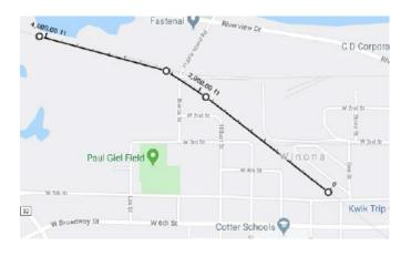
Construct new siding track connecting the main track to the CP Waseca Subdivision over ½ mile east, with power switches and signals, to alleviate congestion west of the Winona Depot.
