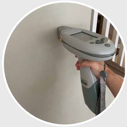
XRF of deteriorated paint
