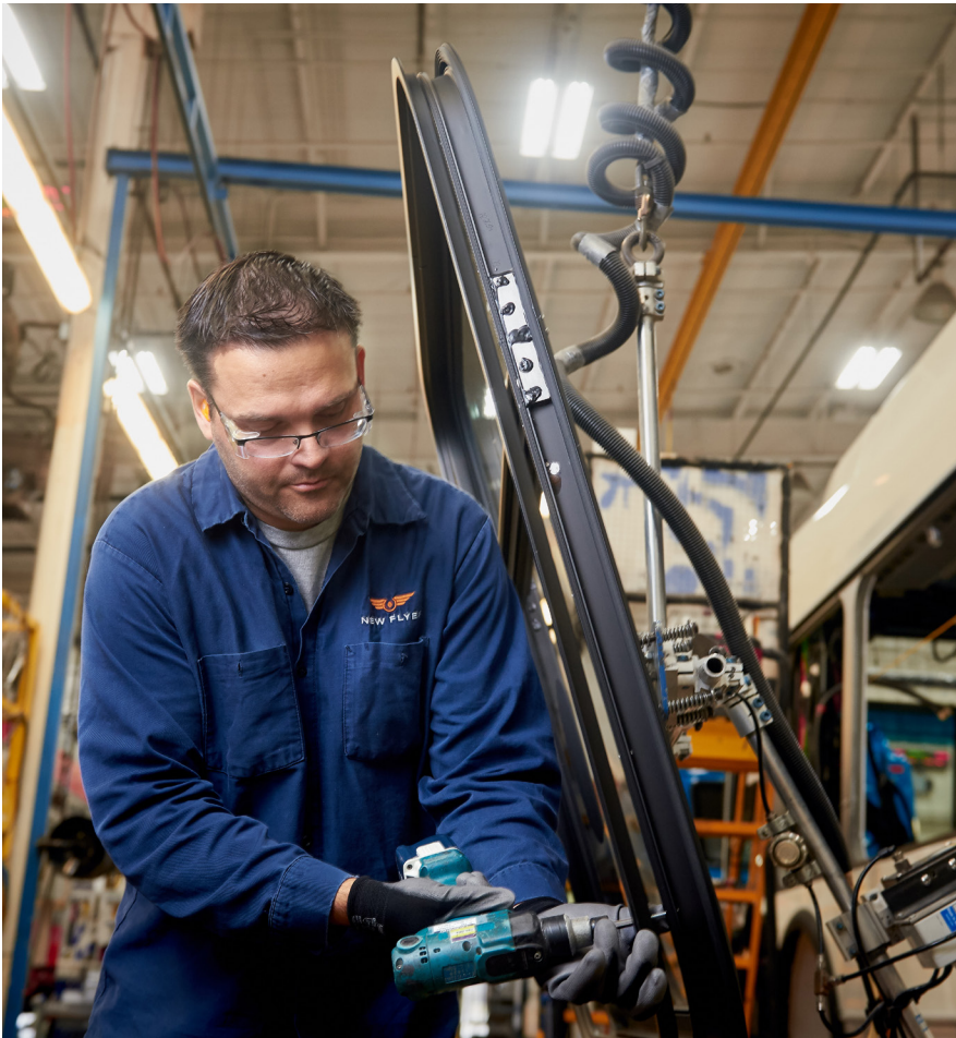
A New Flyer employee works on a window assembly for a new bus. Photo courtesy of New Flyer of America.
