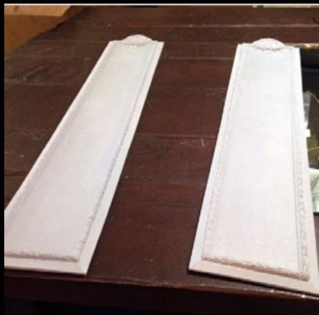
Willamette Hardware, working through Minnesota-based Kendell Doors and Hardware, Inc., began the replication process by creating resin-based molds using the original Capitol hardware as templates.
