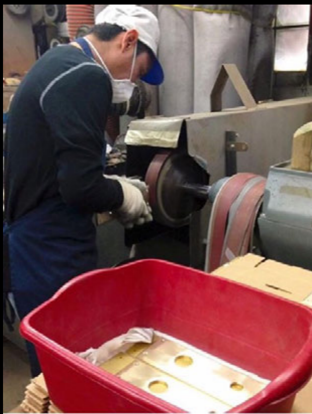
The new metal castings were then shipped back to Willamette Hardware to go through the refinishing process, starting with smoothing out edges.
