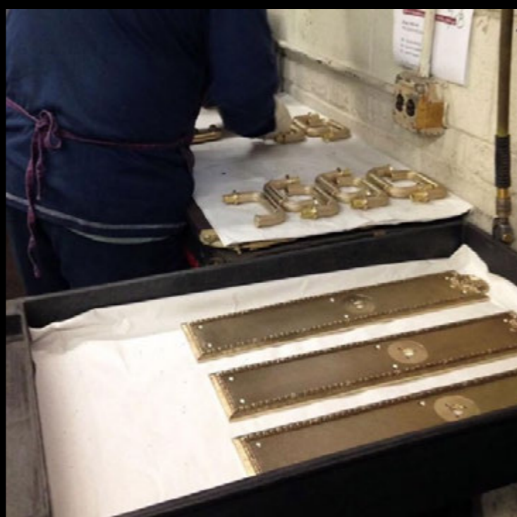
Next, the molds were shipped to a foundry where metal castings were made.
