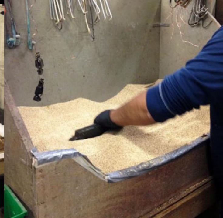
A corn kernal "bath" soaked up any remaining solution on the metal.
