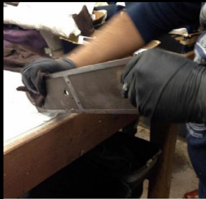
The final step was hand-waxing and polishing. Each piece took about four hours to go through all steps of refinishing.
