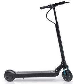
The devices are usually lightweight platforms with two small wheels, similar to a skateboard but with a motor as well as steering and acceleration control via handlebars. Braking is performed through a hand brake on the handlebar or by using a foot-operated rear-wheel brake. Some models have a seat or saddle that sometimes is removable (especially on more powerful and expensive offerings). Many motorized foot scooters weigh around 20 to 65 pounds, although heavier designs are available.
